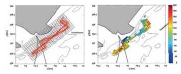
Left: Track of the Navicula during survey for determining the optimal location. Right: Kinetic energy of the current during one tidal cycle (kWh). Black dot: optimal location outside the navigational channel and the envelope of the ferry tracks.
