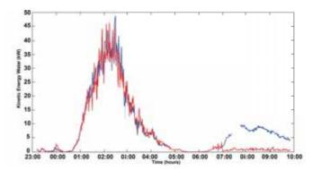
Kinetic energy of the tidal current before and after the turbine that was used in a test phase of the project. Before 7:00, the turbine was not operating. Between 7:00 and 10:00, the blue line indicates the undisturbed flow and the red line the kinetic energy in the flow after extraction of the energy by the turbine.
