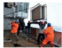
Recovery of the Ultra Clean water sampling system in the Arctic.
