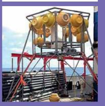
Bottom currents measured by the BOBO (BOttom BOundary) lander are used in model predictions of the dispersion of sediment plumes generated by mining.
