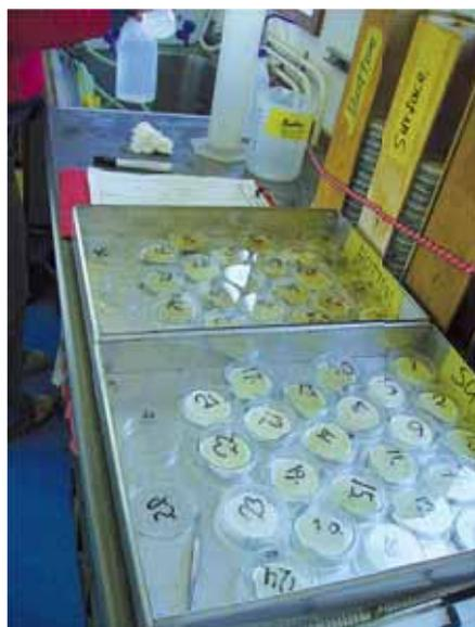
Filters containing sediment collected for the calibration of the TSM-backscatter relation.
