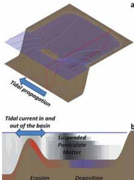
Fig. 2. a) An idealised model set-up of a barrier-island coastline: A tidal wave propagates along the open end of the domain, creating a tidal current in and out of the basin behind the island. b) The strong current results in sediment being eroded from the inlet and transported into the basin, where it is deposited.
