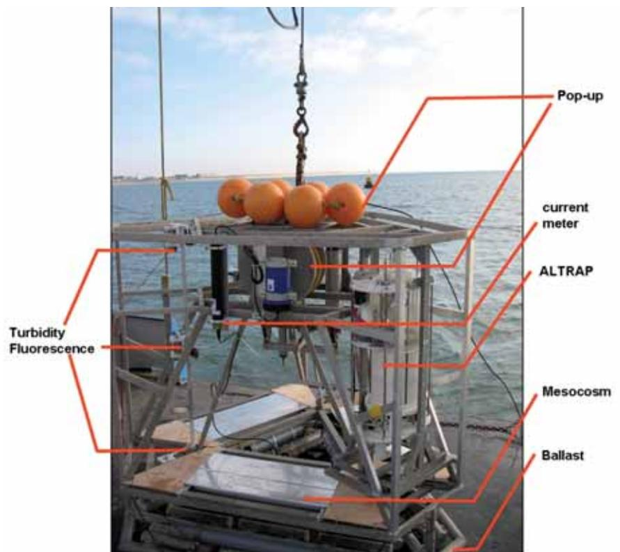
Fig. 1. Overview of one of the lander frames used in the environmental monitoring off the coast of Egmond in 2011.
