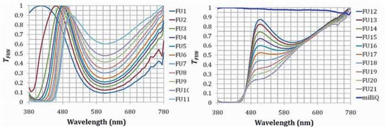
Fig. 3. The normalised transmission ( $T_{FUN}$ ) of the 21 FU-tubes plus an extra tube containing purified water (bold blue line, milliQ).
