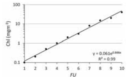
Fig. 4. Chlorophyll concentration as a function of *FU*-number. The *FU*-numbers were derived from the Ecolight RRS spectra. Chlorophyll was varied from 0.1 to 40  $\text{mgm}^{-3}$  with a resulting span of *FU*1 to *FU*10.
