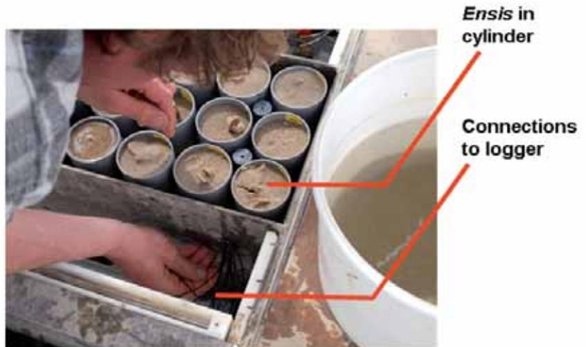
Fig. 2. Placement of sediment cores with live *Ensis* connected to a valve monitor in one of the trays which are mounted on the lander.
