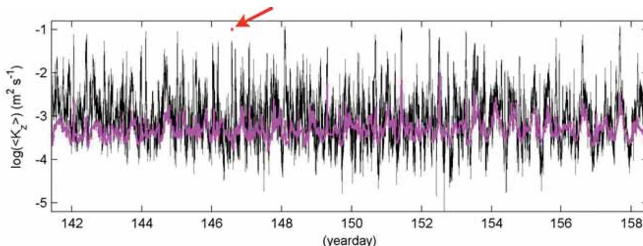
Fig. 2. Total time series of vertically averaged variables using 0.01-Hz data (data points every 100 s). Mean  $\langle K_z \rangle$  (black), with for comparison mean inverse stratification (purple; arbitrary logarithmic scale). The short period including the front of Fig. 1 is indicated by the red dot.
