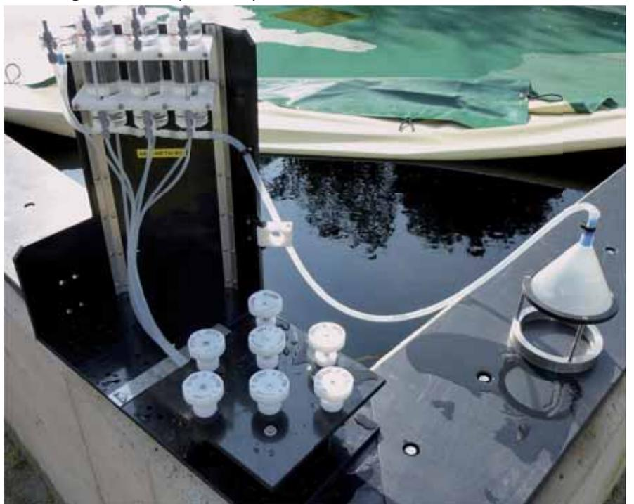
ROV gas sampler during trials in the test basin.
