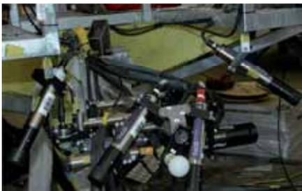
An array of sensors that will move up and down with the tide to attain a constant monitoring depth below the sea surface
