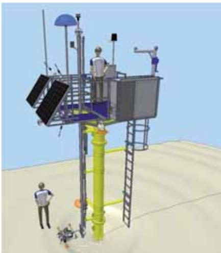
IN PLACE Wadden Sea observatory with solar panels, instruments and cabinets for control units and batteries
