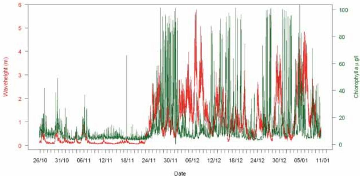
Fig. 3. A record of measured wave height and chlorophyll concentration at 30 cm above the seafloor off the coast of Egmond at 11 meter water depth. Wave events cause an increase in average chlorophyll contents of the near bottom water layer. Especially shortly after the first severe winter storm at the end of November with windspeeds of up to 80km/hr and waveheights up to 3 meter.
