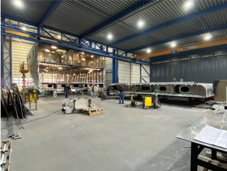
*Ring sections 30 and 40 (left) and bottom section 320 (right). Section 320 is being built upside-down, and will be rotated for attach ring 20 to rings 30 and 40.*
