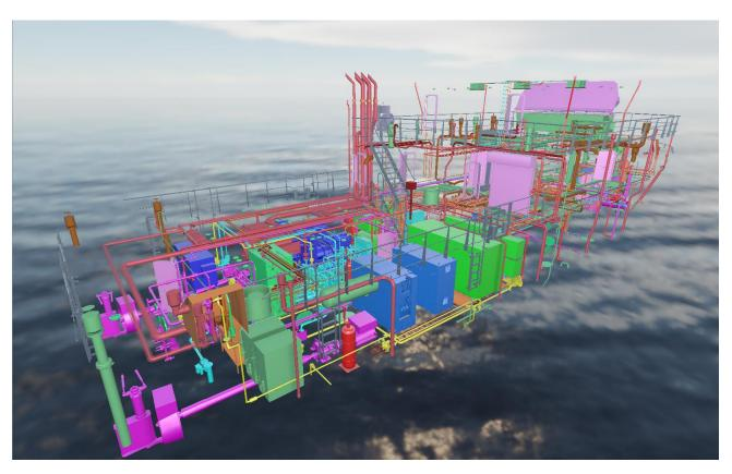
Design of the RV Wim Wolff, with an overview of the pipelines, including fuel (pink), lubricant (dark red), bunker oil (orange), coolant (green), compressed air (light green), exhaust (red), ballast (blue), bilge (yellow), living seawater (dark green), ventilation (matte red), level (light green).
