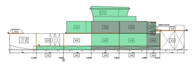
State of affairs in late March. The RV Wim Wolff's hull sections, with the completed sections shown in dark green and the sections still under construction in light green. ©FH
