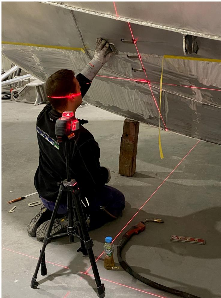
*Applying the draught markings to the hull of the RV Adriaen Coenen. Red lines are laser beams used to align the markings.*
