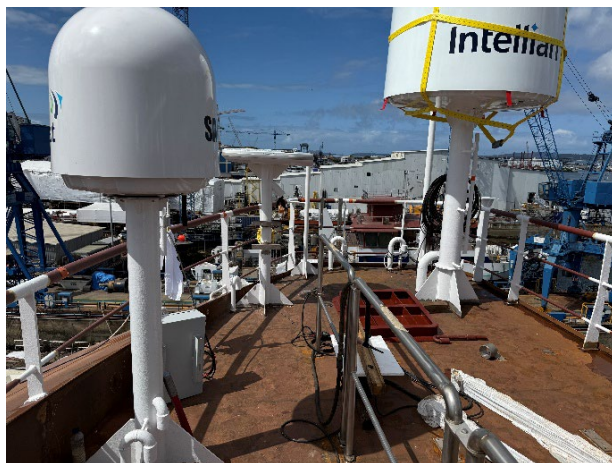
Top deck with Inmarsat communication equipment, navigation antennas and TV dome
