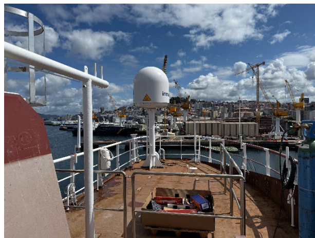
Top deck with Inmarsat communication equipment, navigation antennas and TV dome
