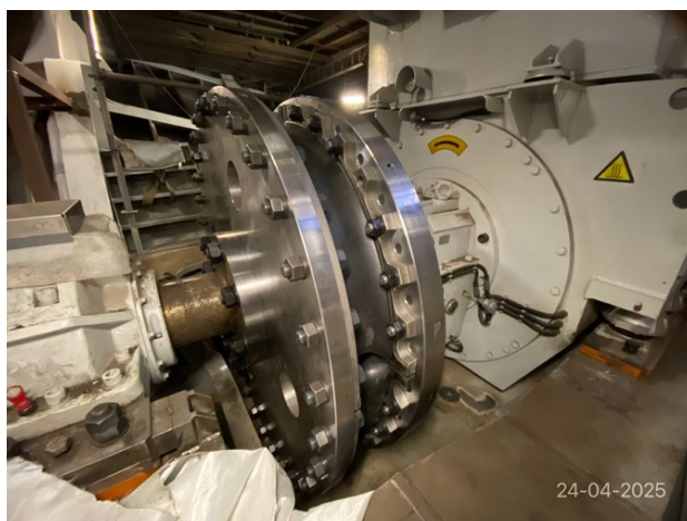
Flexible linkage between the engine and drive shaft has been installed.
