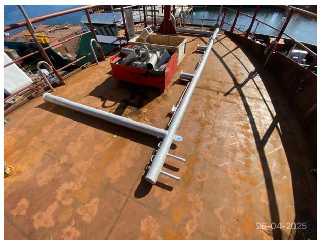
Finishing details top deck Extra rack for future antennas, and dust catcher mount
