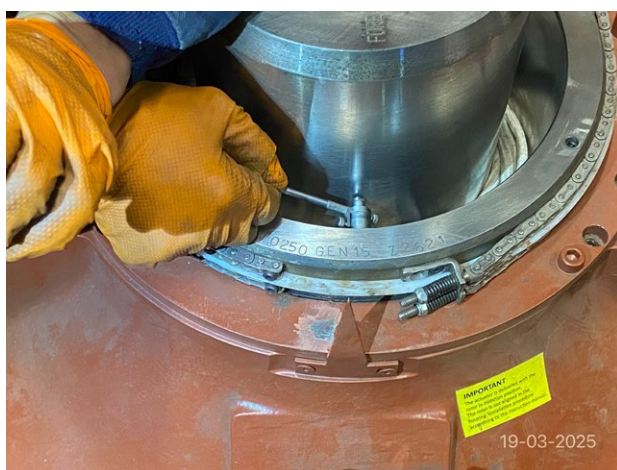
Alignment of rudder stock in the steering gear after casting.
