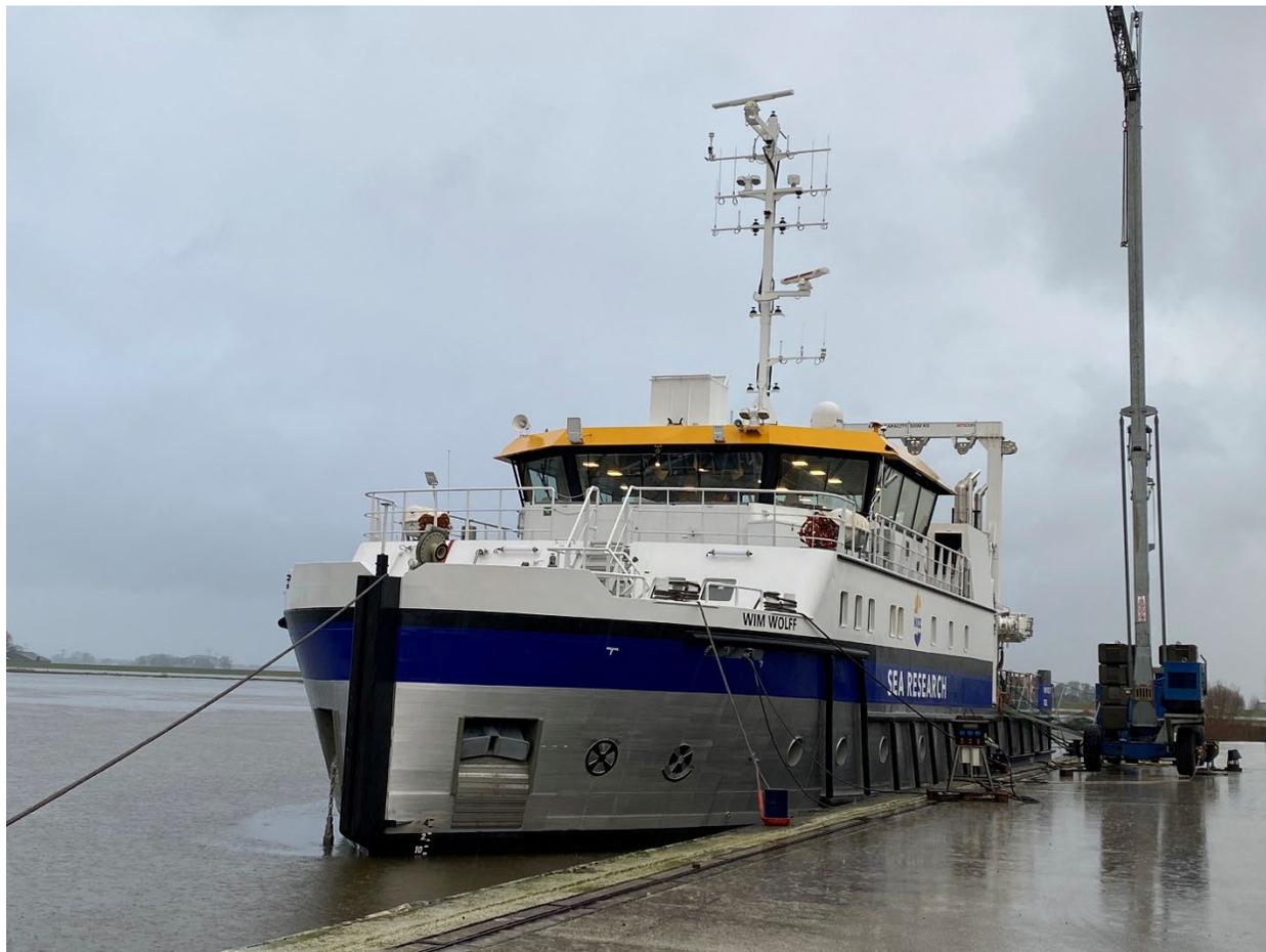
*The RV Wim Wolff at the Tecla Bodewes Shipyards finishing wharf in Kampen, showing the collapsible mast erect and the birdwatching post topside.*
