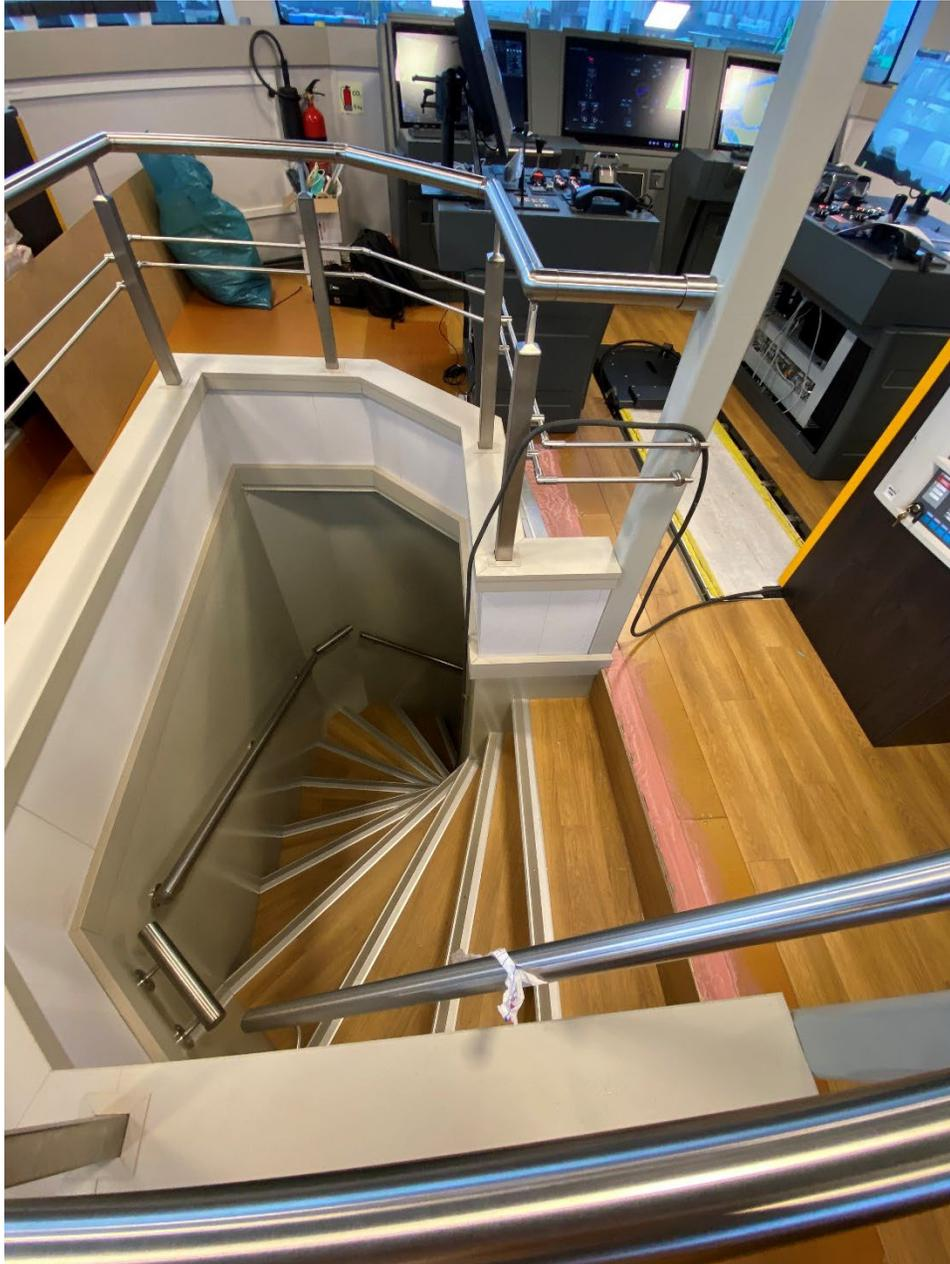
*The ladderway, with wood-effect vinyl deck covering, viewed from the wheelhouse deck. For fire safety reasons, the ladderway is made of steel rather than aluminium.*
