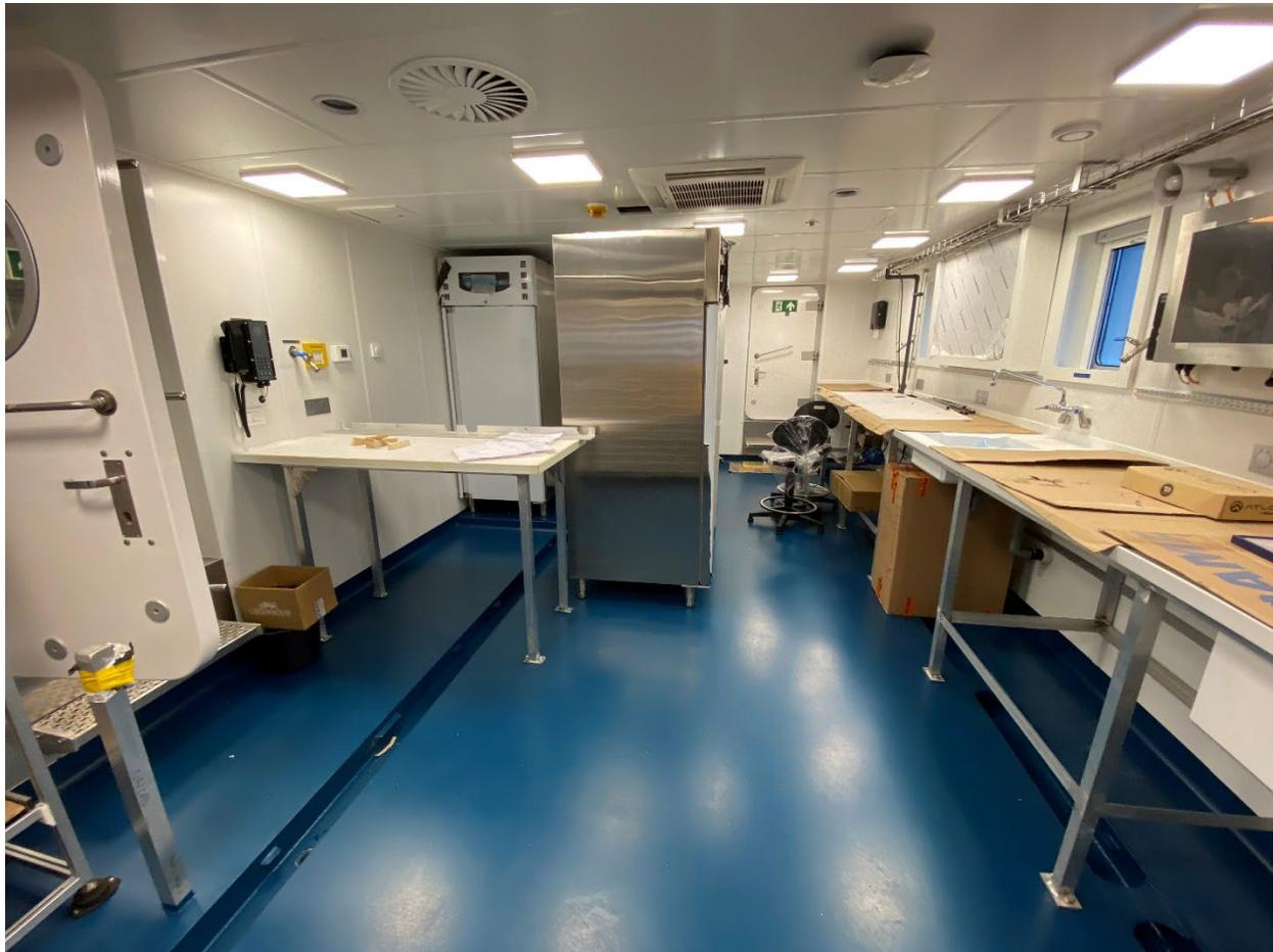
*The wet lab, looking forward. The water-tight hatch to the cabins is visible to the left, work tables to the right, and the refrigerators and freezers for scientific samples in the middle of the lab. The poured floor coating is coloured blue.*
