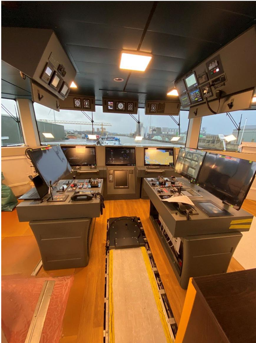
*View of the wheelhouse from aft, showing central control panels equipped with nautical and operating equipment. The black panel in the middle is where the skipper's seat will be attached.*
