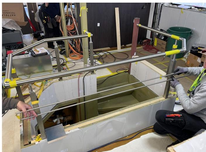
*Mounting the handrail to the wheelhouse ladderway. ©FH*
