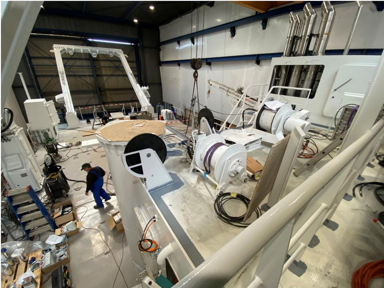
*Top view of the CTD winch, which is connected to the starboard J-frame, but can also serve the A-frame.*
