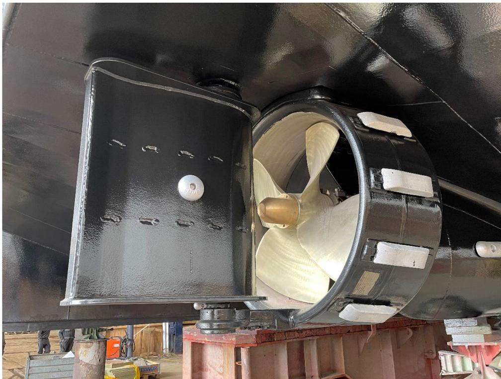
*Sacrificial anodes on the rudder, the propeller duct and drive shaft, and the hull. To function correctly, these anodes must remain untreated (unpainted), so they can 'sacrifice' themselves to preserve the rest of the components. ©FH*
