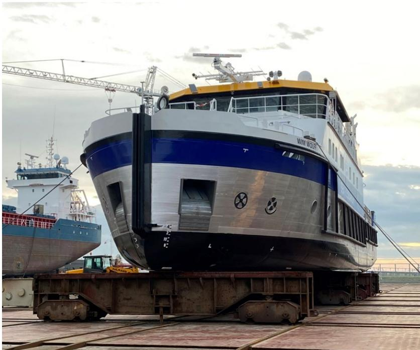
*The RV Wim Wolff rolled outdoors on wheeled carriers.*
