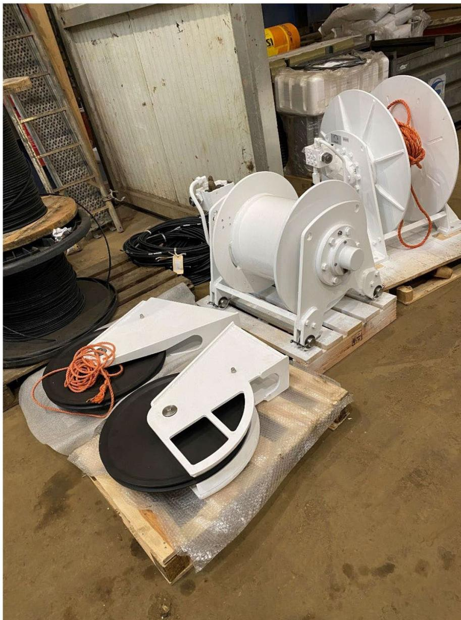
*The guide blocks and (CTD) winches for the A-frame and J-frame are standing by for assembly. The blocks and winches were designed and built especially for the RV Wim Wolf.*
