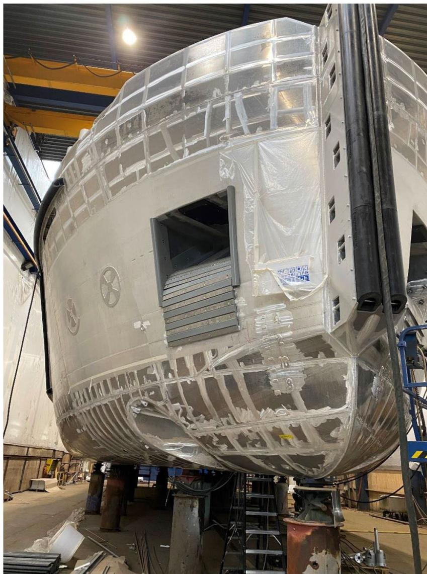
*The starboard bow, with protective strips visible below the fairhead shaft.*
