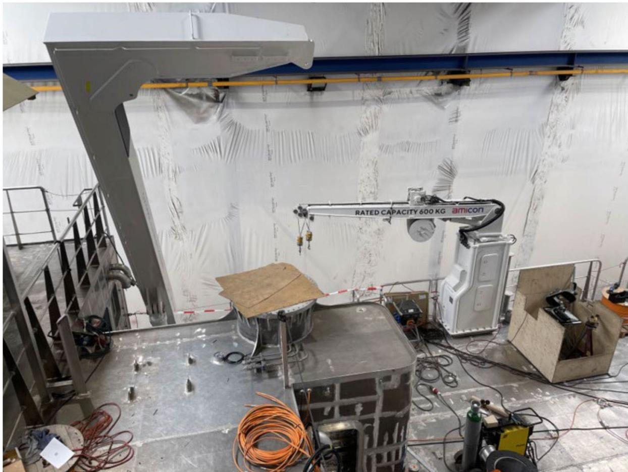
*View from above, with J-frame to the left and the starboard deck crane next to it. ©FH*
