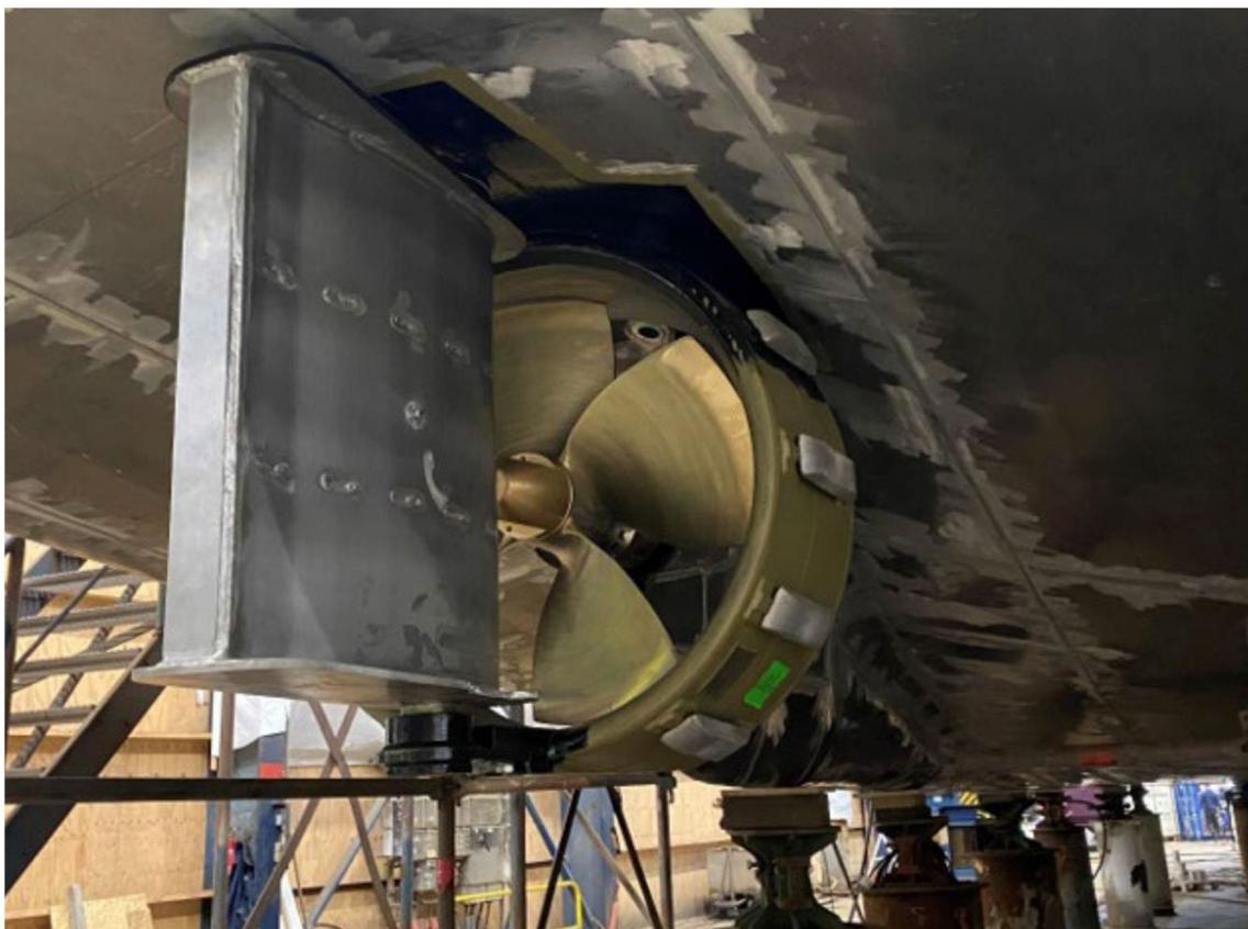
*The rudder mounted behind the propeller in the duct. Sacrificial anodes, visible on the propeller duct, will help protect the propeller and duct from corrosion.*
