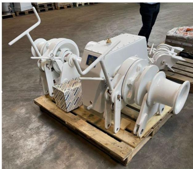
*The anchor gear in the production facility, awaiting assembly. ©FH*
