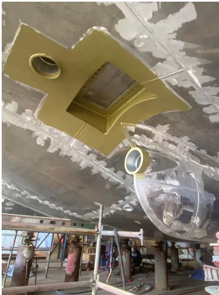
*One of the stern tubes below the RV Wim Wolff following the boring work. The protective paint system has been applied in preparation for the installation of the drive shaft.*
