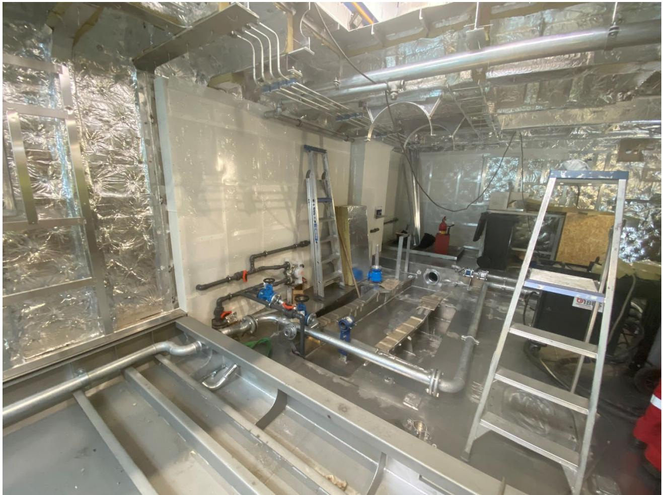
*The engine room, showing the base fittings for the engine and the bored port for the stern tube. The base fittings for the battery room are visible in the foreground.*
