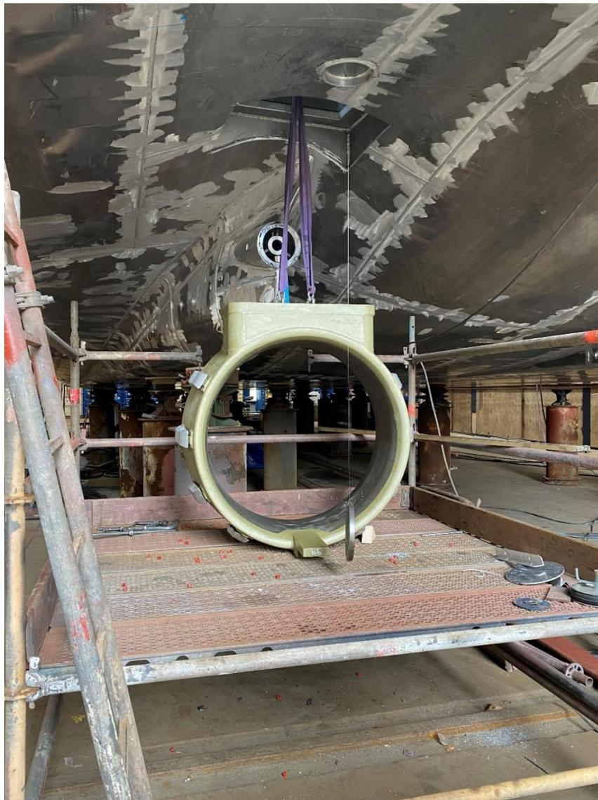
*One of the two stern tubes, with the propeller tunnel in the foreground ready to be lifted into position.*
