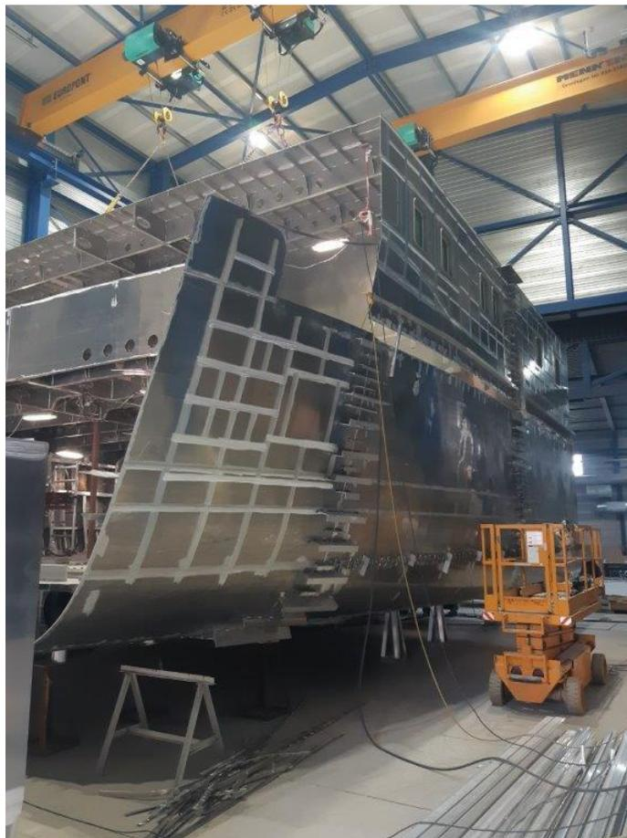
*State of affairs in late March. The first bottom sections (400 and 300 sections) have been positioned together, and the first superstructure section (200 section) has been installed. ©PB*
