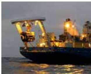
Recovery of ROV ROPOS after one of its 12 dives to the southern Central Indian Ridge during the BGR cruise. During the dives, ROPOS spent up to 8 hours on the sea floor at a depth of up to 3400m and collected rocks, sediments and biological samples from active vent sites. [www.ropos.com](http://www.ropos.com)
