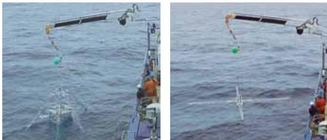
*The unfolding of the five-line 3D mooring.*
