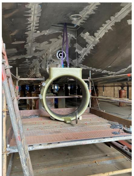
One of the two stern tubes, with the propeller tunnel in the foreground ready to be lifted into position.
