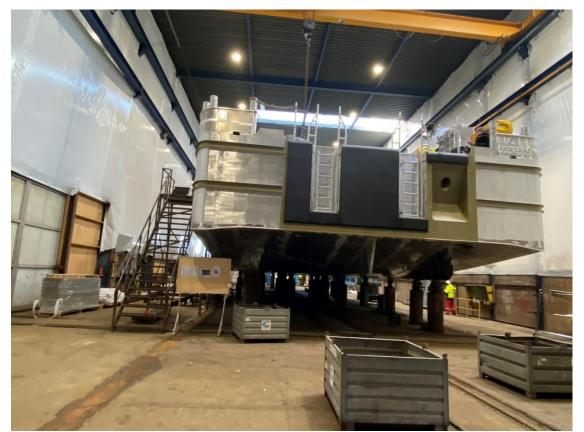
The hull at the TBSY final construction facility, showing the ladderway moved to the port side. The aft section is starting to take on its final form.
