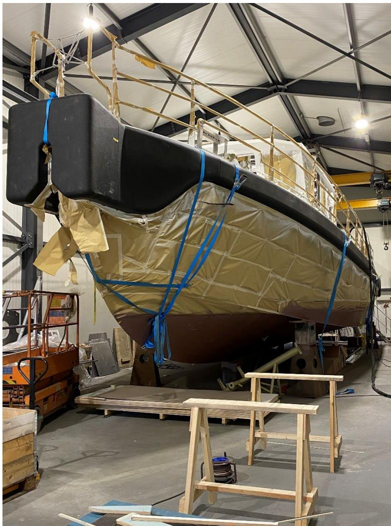
*State of affairs in late April. The first layers of the paint system have already been applied. Areas of the hull that will not be painted have been masked off. The protective bumper has also been fitted to the bow push head.*
