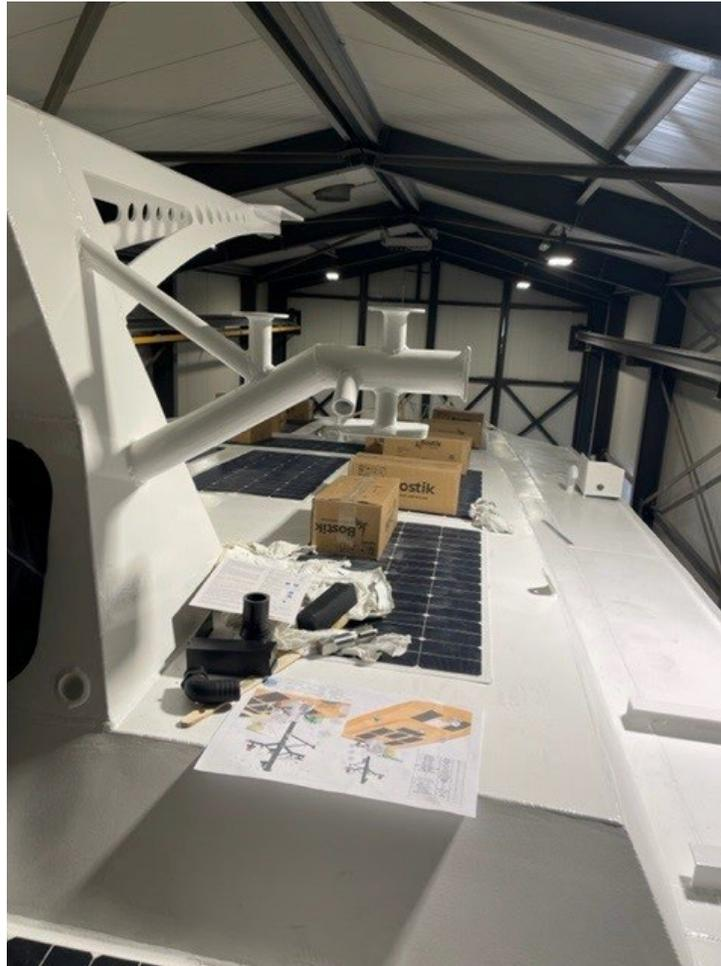
*The solar panels on the wheelhouse roof ©FH*
