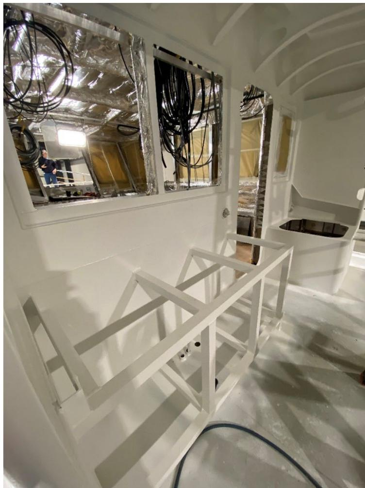
*The wet lab frame aft of the wheelhouse.*
