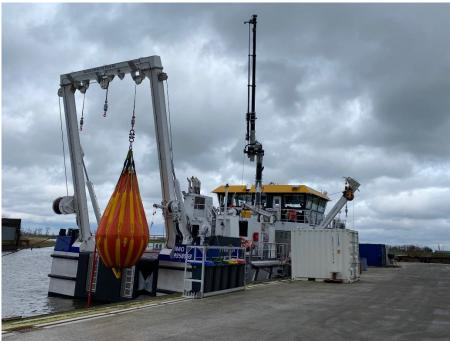
Load check and test of the A-frame and winches, using a water-filled bag.
