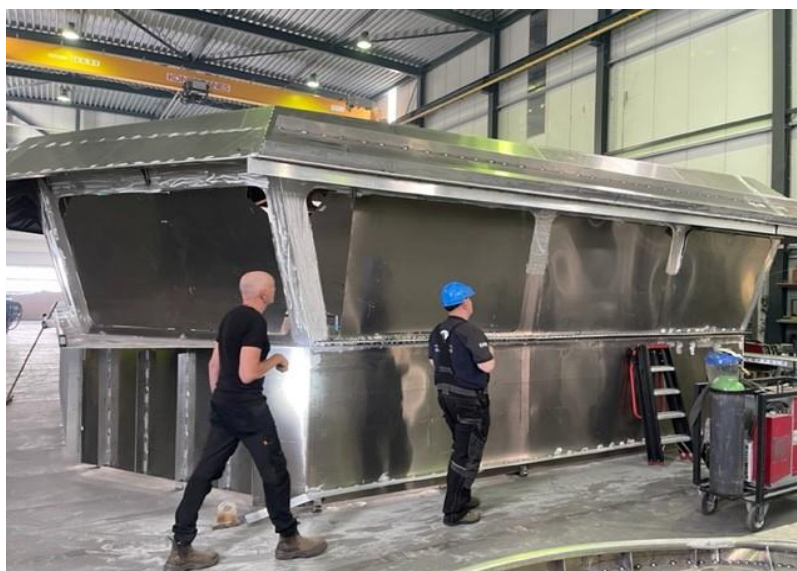
The wheelhouse section (270) is nearing completion.
