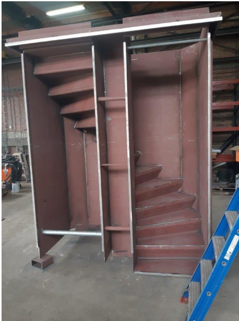
The first section of the ladderway is ready for installation. The colour of the metal shows that the ladderway is made of steel, rather than aluminium.
