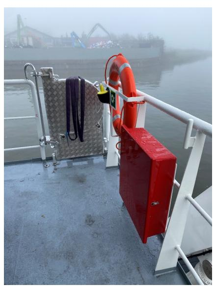
Firefighting equipment and lifebuoy shown on the starboard bridge deck. The platform connecting to the gangway is shown in the stowed position.
