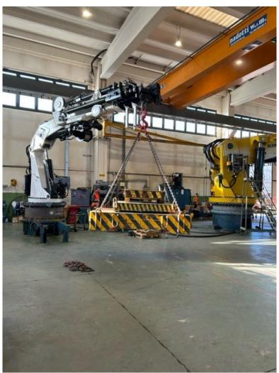
Functionality tests on the Heila deck crane at the manufacturer in Italy. ©TBS
