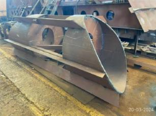
Bow thruster tunnel built to size
