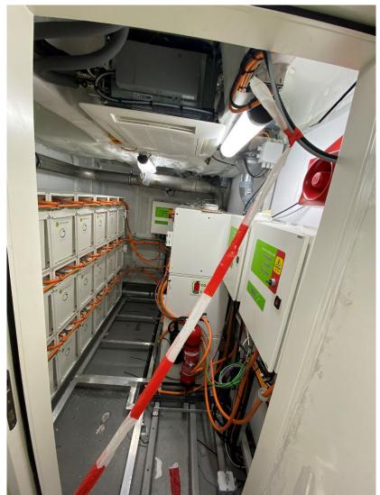
The batteries can power the vessel at night while it is on station and not underway.
