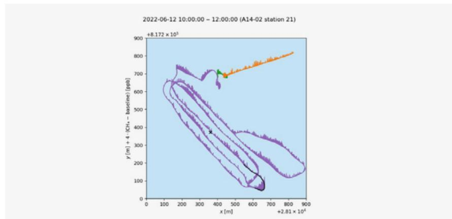
**Figure 8-9:** Concentration  $CH_4$  and  $C_2H_6$  measured by using the SLURF and the membrane, around A15-03 (pointed with x).
