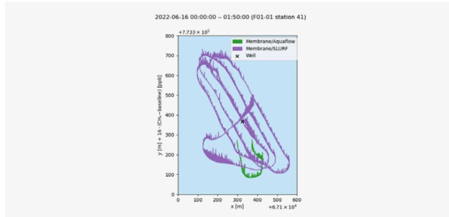
**Figure 8-18:** Concentration  $CH_4$  and  $C_2H_6$  measured by using the SLURF and the membrane, around B13-01 (pointed with x).
