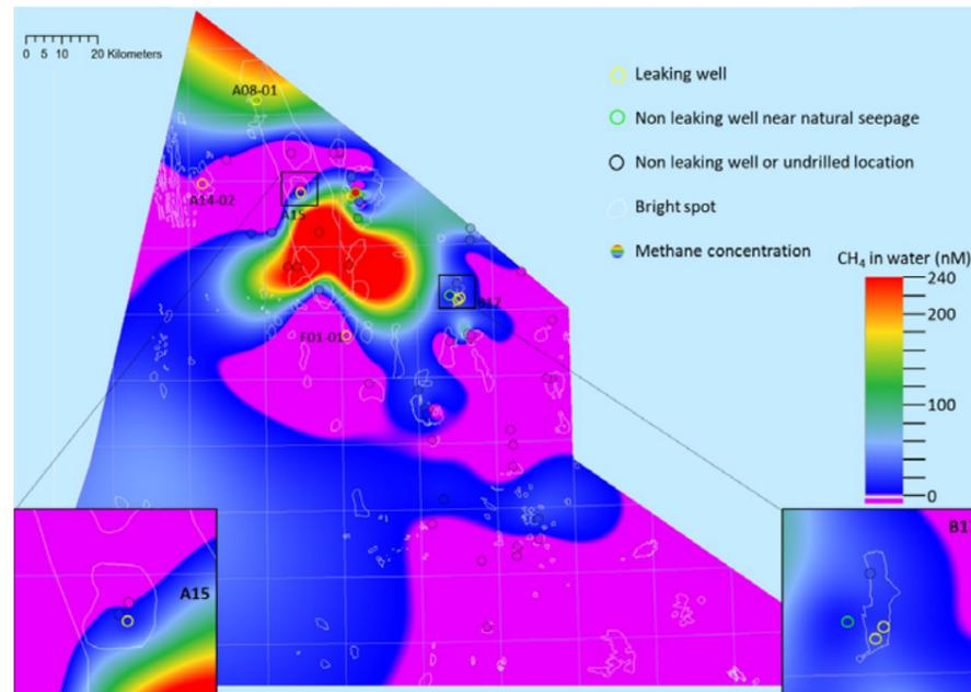
**Figure 10-7:** Methane concentration in the water (dots) compared to the water depth (map). Note that the 6 locations in the shallowest part (Doggerbank) are all below the detection limit (black), while the higher methane concentrations are found to the south of the Doggerbank. The Doggerbank could act as a barrier for dissolved methane.
