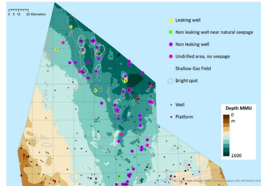
**Figure 10-8:** Relation between the depth of the MMU (Base of the Upper North Sea Group) and leaking wells. The depth of the MMU is a proxy for its thickness.
