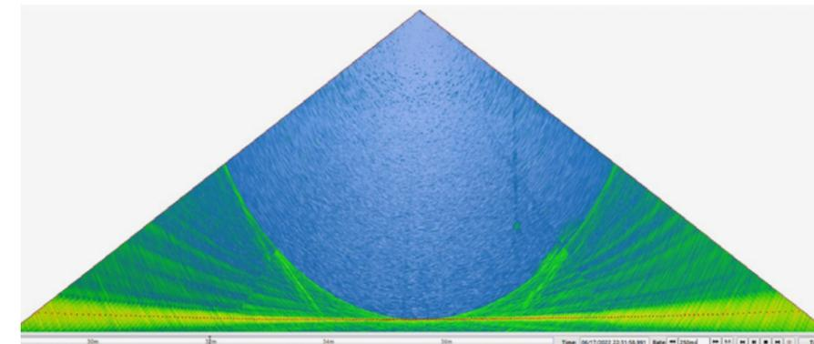
**Figure 3-4:** The bubble plume source at B17-03 is very hard to see, since it coincides with the side lobe of the first seabed reflection.
