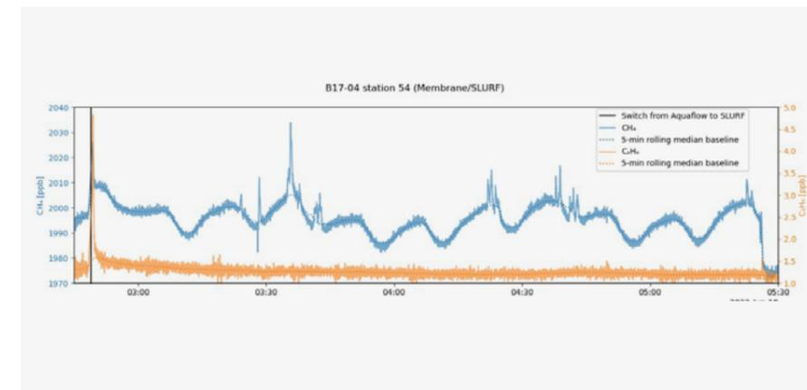
**Figure 8-22:** Concentration  $CH_4$  and  $C_2H_6$  around B17-04, with the peaks on top of the background atmospheric concentration showing  $CH_4$  enhancements.
