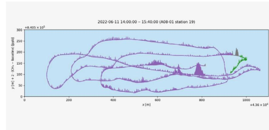
**Figure 8-5:** Concentration CH<sub>4</sub> plotted at the track. Every ppb at the baseline is projected as 2m.
