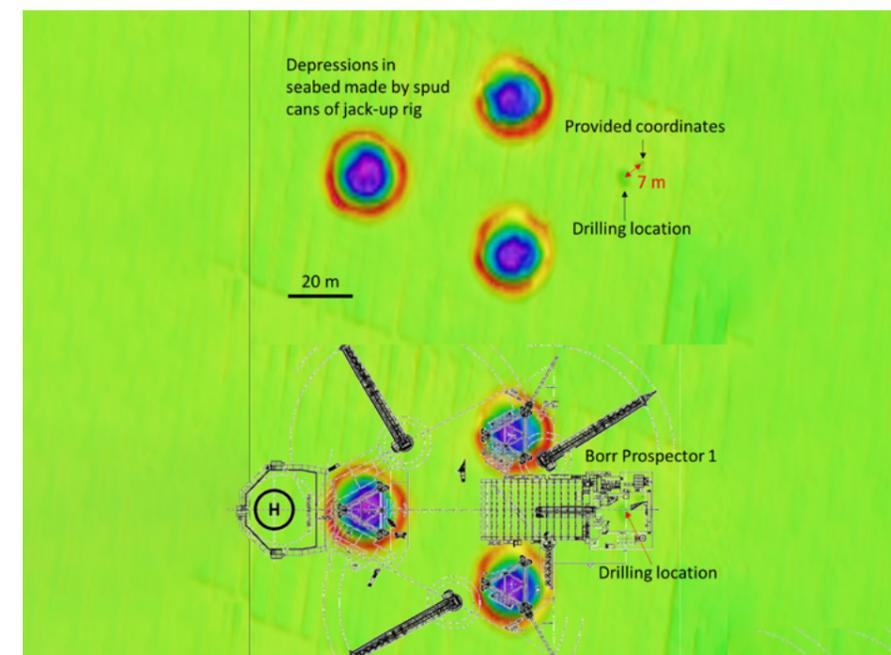
**Figure 2-2:** (Top) At well F05-06 the impressions of the legs of the jack-up rig are still visible as depressions in the seabed. (Bottom) When the plan view of the jack-up rig used for drilling this well is projected over the depressions, we find that a depression in the seabed lines up with the location of the drilling string. This drilling location is 7 m from the well coordinates provided by the operator.
