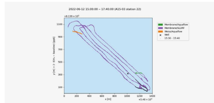
**Figure 8-12:** Concentration  $CH_4$  and  $C_2H_6$  measured by using the SLURF and the membrane, around B17-3 and B17-05 (pointed with x).
