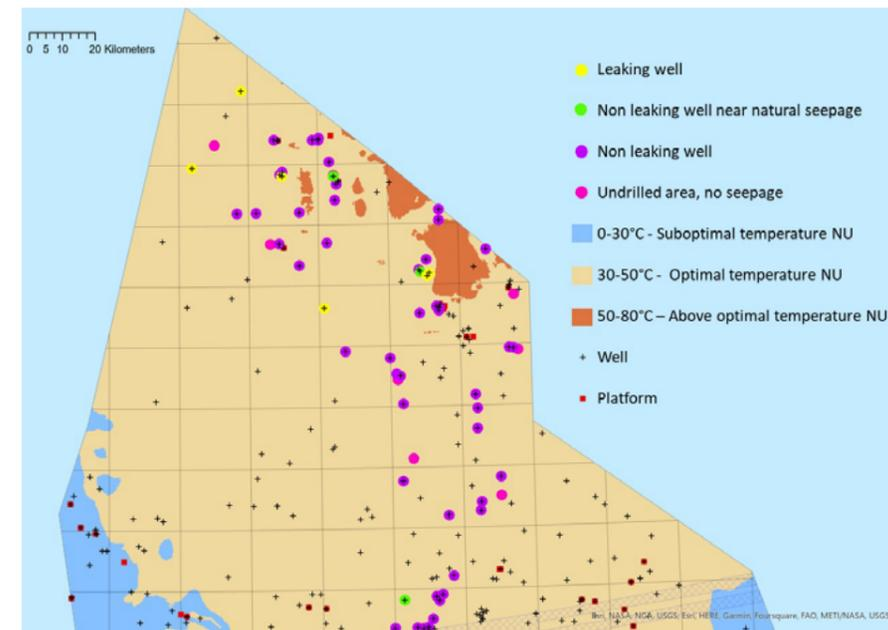
**Figure 10-9:** Relationship between the temperatures within the Upper North Sea group and well leakage from shallow gas. Note that all presumed to be leaking wells are found close to the region of above optimal temperatures for biogenic gas generation. Source: <https://www.geodeatlas.nl/>
