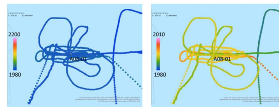
**Figure 9-4:** Methane concentrations around the A08-01 well are not varying a lot over time. Left: methane concentrations with the color bar scaled to the long term maximum and minimum of the methane concentration. Right: the same methane concentration data with the color bar scaled to the data range around A08-01. Note that the methane values are very slowly changing and only about 15 ppm.
