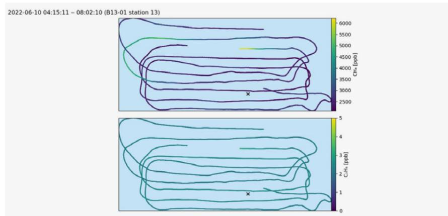
**Figure 8-19:** Concentration  $CH_4$  and  $C_2H_6$  around B13-01, with the peaks on top of the background atmospheric concentration showing  $CH_4$  enhancements.
