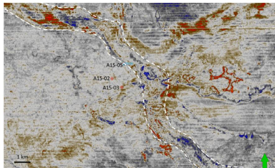
**Figure 7-2:** Seismic section through wells A15-05 and A15-03. Since A15-05 is a recent well, no well trajectory information is present. The well is located at the edge of a tunnel valley.
