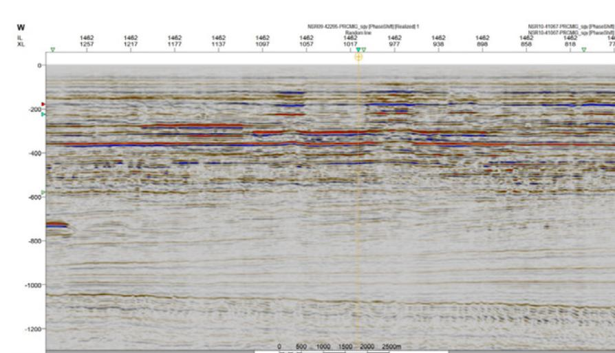
**Figure 4-4:** Seismic profile through well A14-02 (Amber).
