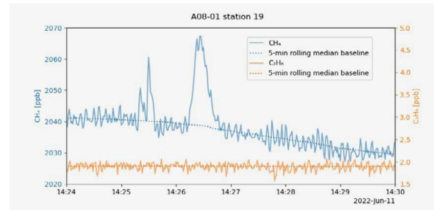
**Figure 8-4:** Zoom in on the plumes of CH<sub>4</sub> on top of the atmospheric background at A08-01.
