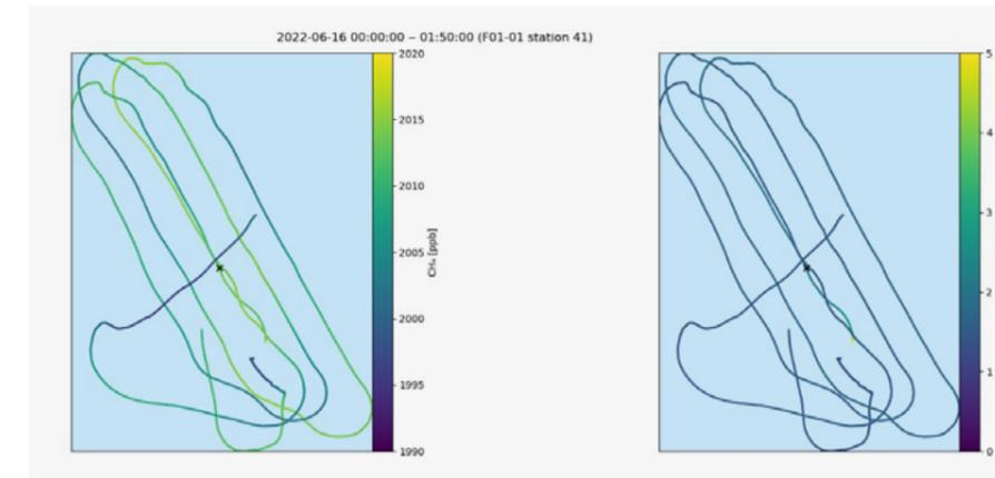
**Figure 8-16:** Concentration  $CH_4$  and  $C_2H_6$  around F01-01, without peaks on top of the background atmospheric concentration indicating no  $CH_4$  enhancements.
