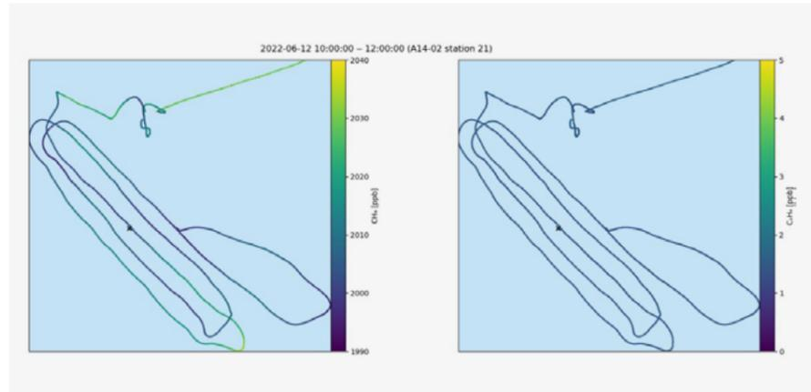
**Figure 8-7:** Concentration  $CH_4$  and  $C_2H_6$  around A14-02, with the peaks between 10:47 and 10:50 showing  $CH_4$  enhancements.
