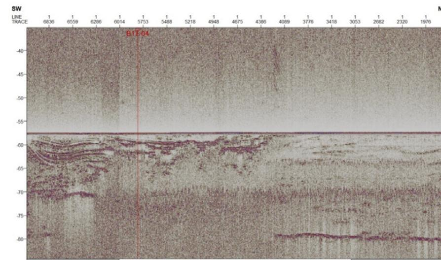
**Figure 6-2:** SBP data at well B17-04. No bubble plume is present at the wellhead, but one can be seen North-East of the well between traces 4386 and 4089. Around the well, a channel complex is present. Peat is not identified in this profile.
