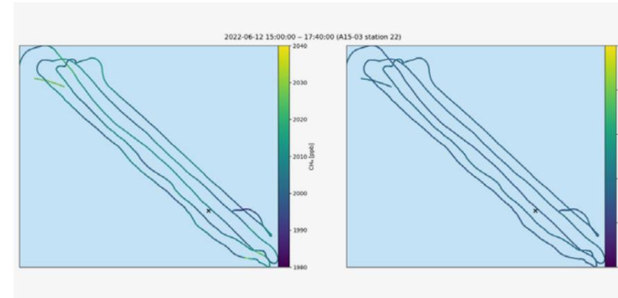
**Figure 8-10:** Concentration  $CH_4$  and  $C_2H_6$  around A15-03, with the peaks on top of the background atmospheric concentration showing  $CH_4$  enhancements.
