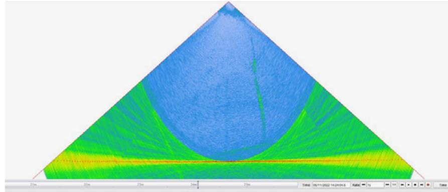
**Figure 3-2:** At the wellhead of A14-02 a bubble plume was found.
