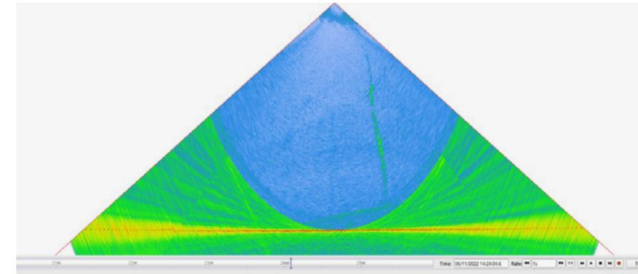
**Figure 3-5:** At well B17-05 a very large bubble plume was observed.
