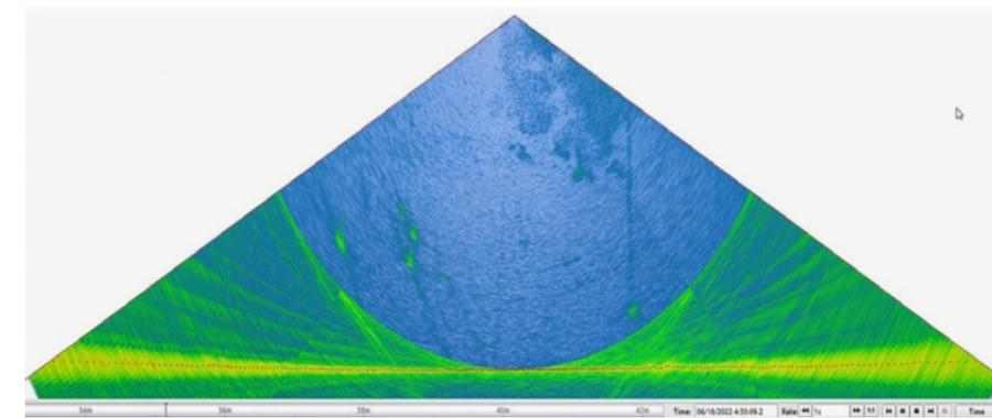
**Figure 3-10:** Bubble plumes at in the vicinity of well B17-04. At the well itself no bubble plume was found. Note that the SLURF, a hose with depressor weight used for pumping up water from near the seabed, is visible on the right.
