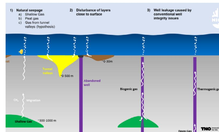
**Figure 1-1:** Sources of biogenic methane and leakage mechanisms for biogenic and deep (thermogenic) gas. Potential leakage pathways for existing wells are (a) between cement and casing, (b) between the casing and the cement plug, (c) through the cement, (d) through the casing, (e) through fractures in the cement, and (f) between cement and formation (Celia et al., 2004).
