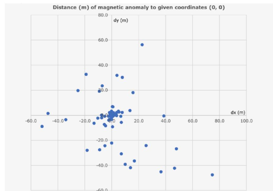
current oblique to the ships heading. For 30% of the wells that were measured by the hydrographic service an offset of more than 15 m was observed (see Figure 2-1). Based on this we concluded that a significant number of wells could potentially have an error in the reported position and a recalibration would be needed during the measurement campaign.
