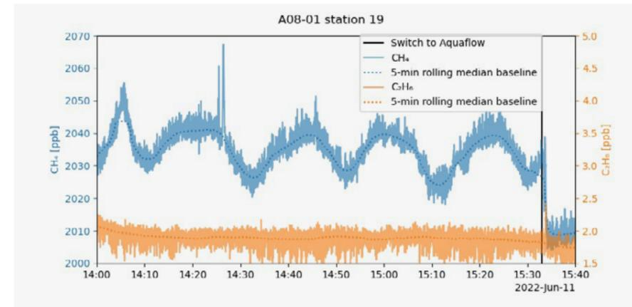
**Figure 8-3:** Concentration CH<sub>4</sub> and C<sub>2</sub>H<sub>6</sub> around A08-01, with the peaks between 14:25 and 14:27 showing CH<sub>4</sub> enhancements. Ethane stays constant, indicating that the bubbles contain no thermogenic gas.
