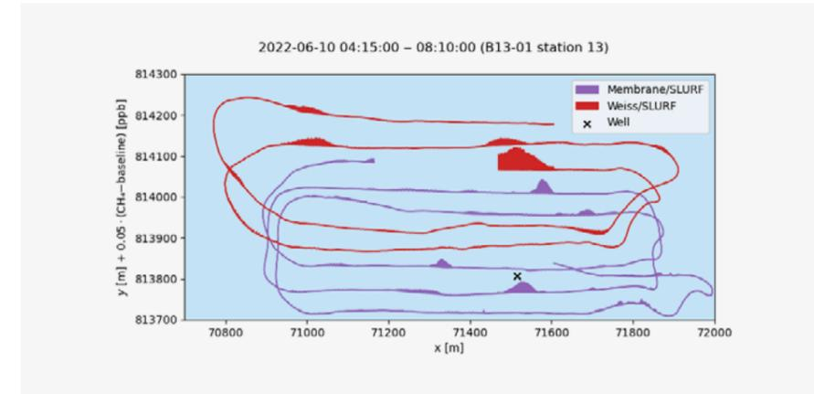
**Figure 8-20:** Concentration  $CH_4$  plotted at the track around B13-01. Every ppb at the baseline is projected as 0.05m.
