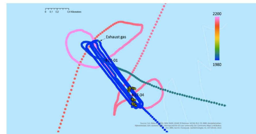
**Figure 9-3:** Methane concentrations were measured twice at B17-01 and B17-04. During the first visit the concentrations were high during the entire visit, and low during the entire second visit. No local elevated methane concentration above the many plumes was detected.
