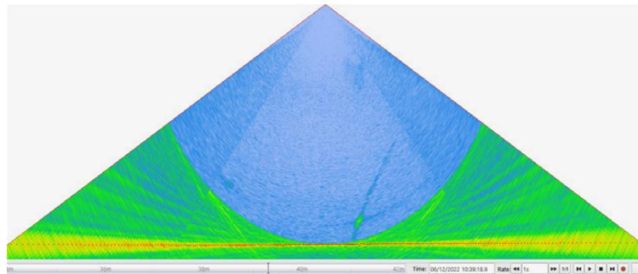
**Figure 3-3:** At the wellhead location of well A15-03 two bubble plumes were observed.
