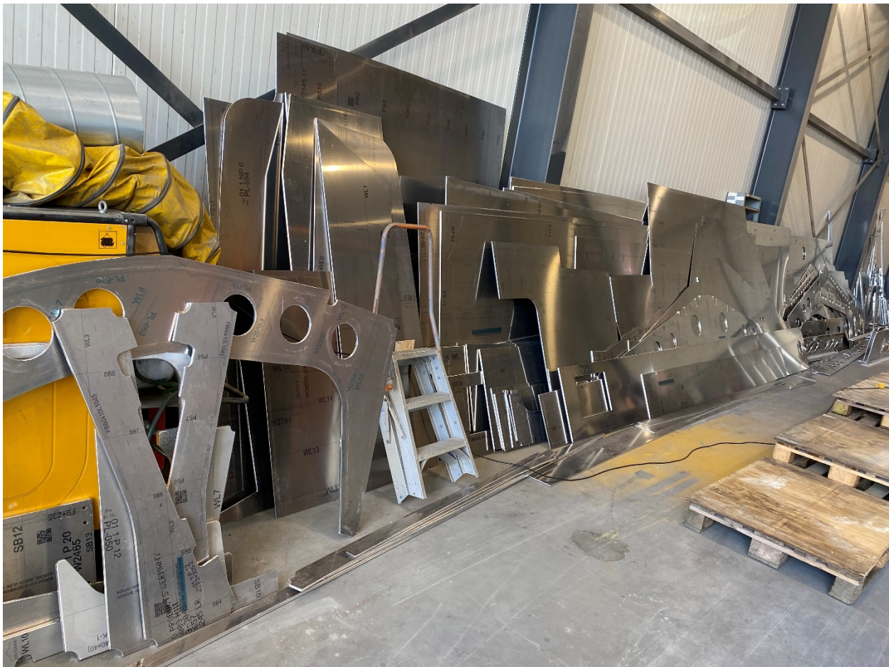
The first aluminium for RV Adriaen Coenen, currently still individual parts, soon a hull
