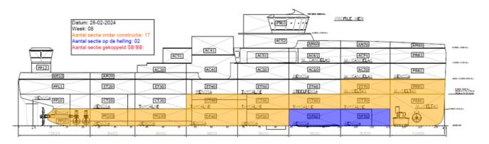
Two double-hull sections are now in their definitive locations in the production facility. The yard is expected to join the next section early in week 10. A total of 17 sections are currently under construction, and various components of other sections are in the pre-production phase.
