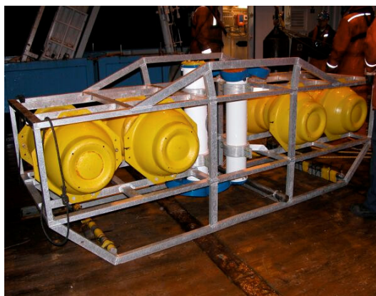
Photo (Erica Koning): Deep-towed body with up- and downlooking ADCP.
