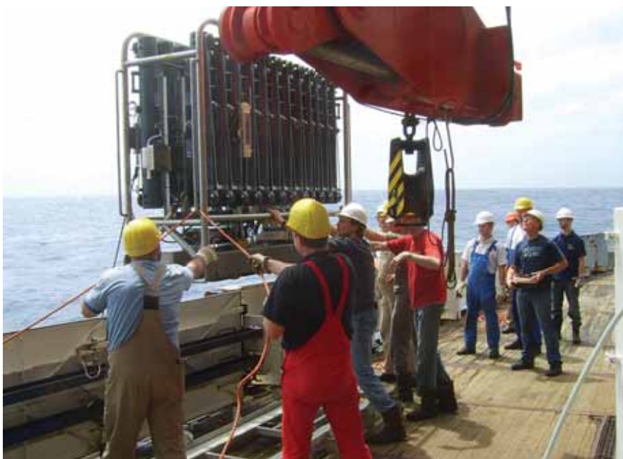
Fig. 2. First deployment of the Titan(ium) ultraclean frame with internal teflon coated PVC water samplers at 11 February at test station (37°S, 13°E) in still warm temperate region. Handling of the frame by ship's crew and NIOZ trace metal scientists; in the background Willem Polman (right) with the remote control leading the operation, next to boatswain Reiner Loidl (left) supervising. See Marine Chemistry (2008), 111, 4-21 for details of Titan system. Photograph courtesy Ilias Nasir.
