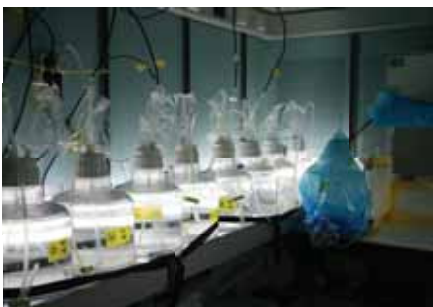
Carbondioxide incubation experiments under controlled laboratory conditions to mimic the effect of CO 2 on the plankton community during the last glacial maximum (190 10 -6 atm), present (380 10 -6 atm) and the future acidified ocean (750 10 -6 atm). This project of the Netherlands Polar Program (NWO) is a collaboration between NIOZ and the University of Groningen (Ocean Ecosystems and Ecophysiology of Plants) on the Southern Ocean in a High-CO 2 World. Shipboard research by Babette Bontes and Ika Neven, photograph by Ika Neven.
