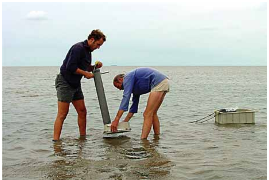
Fig.2. Hand operated core sampling in intertidal areas
