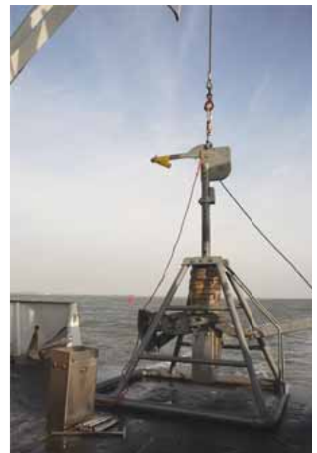
Fig. 3. Box corer for sampling in subtidal areas (photo A.G. Brinkman)
