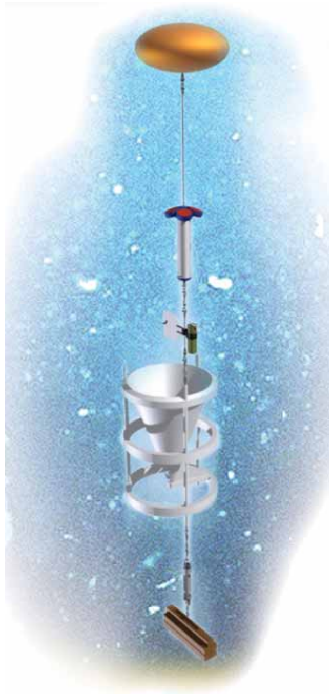
Schematic impression of a mooring. From bottom to top: Iron anchor weight, acoustic release, sediment trap, current meter, Acoustic Doppler Current Profiler (ADCP), and a sub-surface buoy to keep the mooring upright during the measurements and to lift it to the sea-surface after detachment from the anchor weight by means of an acoustic signal from the research vessel.
