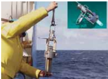
Recovery of the mono-corer during the LOCO-IS cruise. Inset: 3D CAD design drawing of the mono-corer
