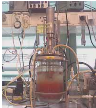
Anammox enrichment sequencing batch reactor, used during the temperature experiment.
