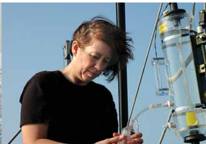
Taking subsamples from a Niskin bottle for analyses of pH and carbondioxide concentrations as part of the JetSET sampling program..
