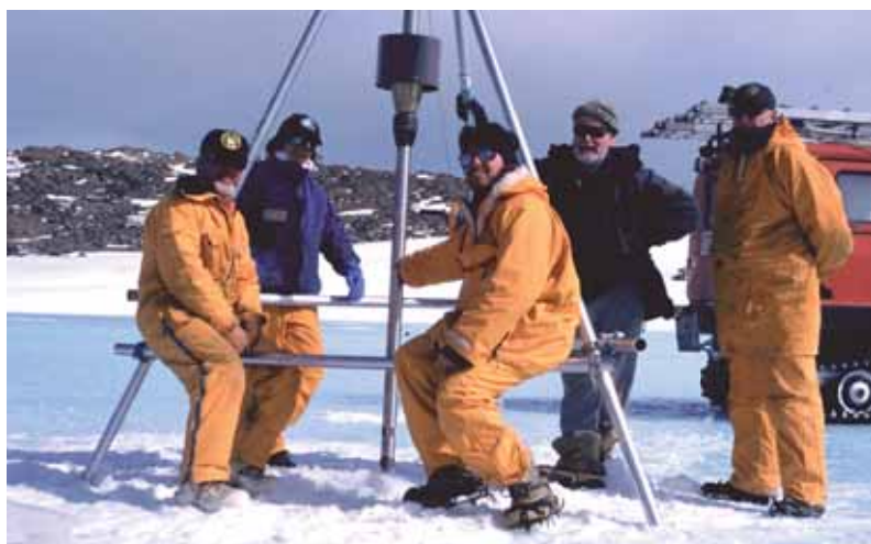
Gravity coring at Ace Lake, Vestfold Hills, Antarctica. The sediment core was 150 cm long, spanning 10,450 calendar years of deposition.
