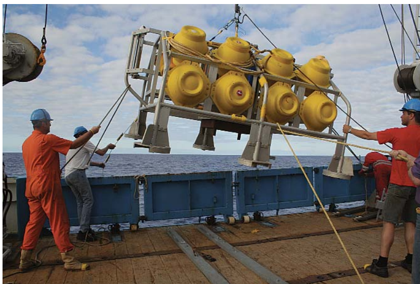
Deployment of LOCO/IW mooring in the North Atlantic Canayr Basin.
