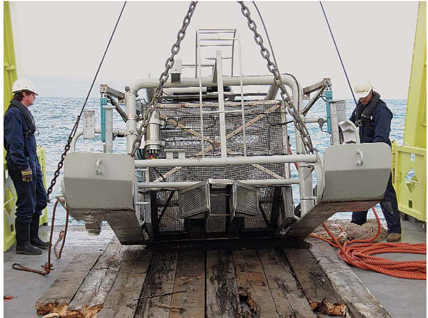
On the Rijkswaterstaat vessel MV Arca NIOZ-technicians deploy the Deep Digging Dredge during a combined BSIK and Marine Protected Areas cruise on the North Sea.
