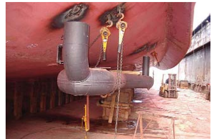
Mounting of the sensor-array under the vessel
