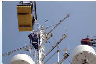
All sensors – in this case GPS antennas - had to be measured within a coordinate system having 1mm accuracy
