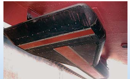
The T-shaped sensor-array mounted in a streamlined gondola under the ship's hull
