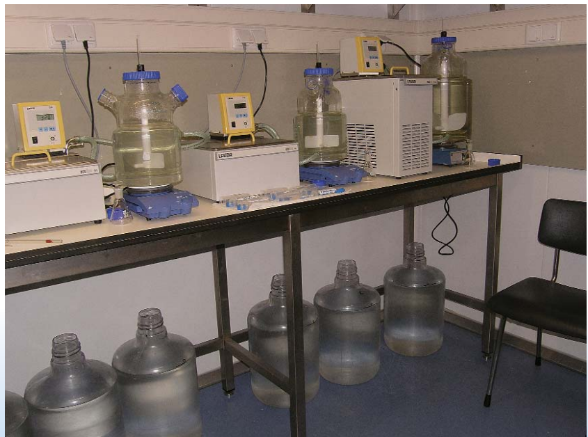
Fig. 1. Set-up of the mesocosm experiments to calibrate the TEX 86 at 30-40°C using waters from around the Seychelles. Experiments were carried out in the dark.
