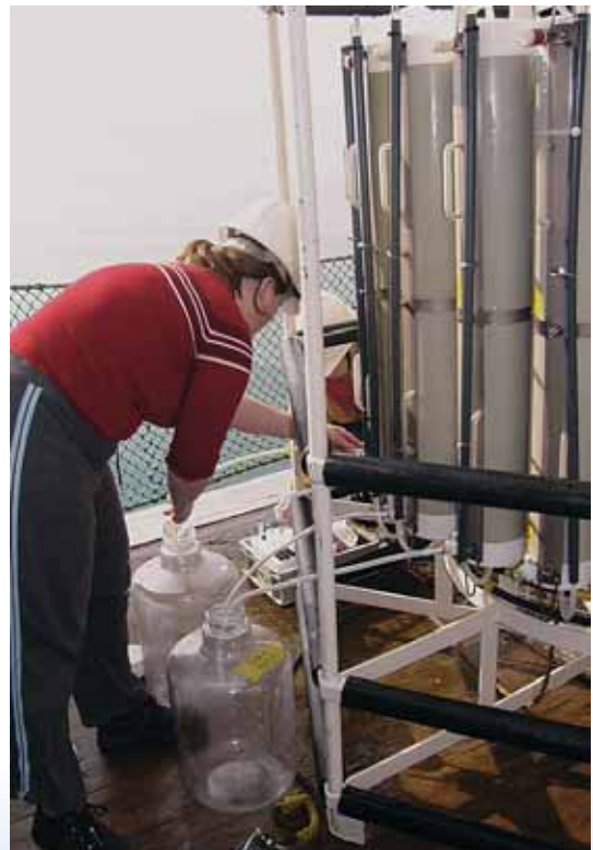
Seawater sampling from the CTD-frame for DNA and lipid analysis on the RV Pelagia.
