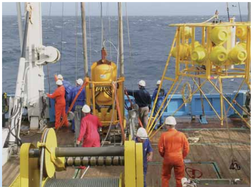
BOBO lander (right) and vibrocorer (left) on deck of RV Pelagia.
