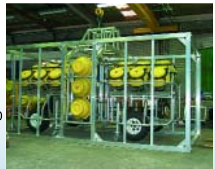
The MOVE mounted in its deployment-frame ready for sea-trials
