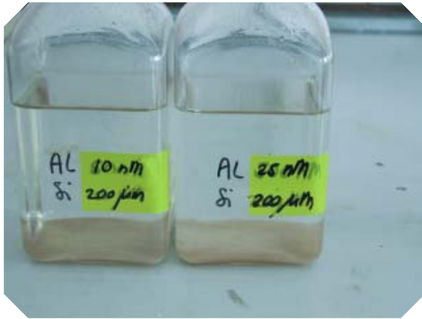
Incubation of diatom frustules of Thalassiosira punctigera in natural seawater at increasing concentrations of dissolved aluminium.
