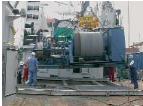
Loading the Towed Ocean Bottom Instrument winch on RV PELAGIA. (photo courtesy SOC)
