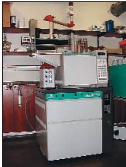
Installed Thermofinnigan Delta PLUS XL stable isotope mass spectrometer with gas chromatograph and combustion/pyrolysis interface for measuring the stable isotopes of individual organic compounds.
