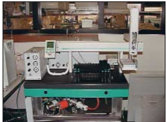
Installed Thermofinnigan Delta PLUS isotope mass spectrometer with GasBench for measuring the stable isotopes of inorganic carbon in seawater and sediments.
