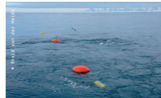
AFTER THE DATA has been collected and the instruments are serviced the LOCO mooring is redeployed in the Irminger Sea and will stay there for some years.
