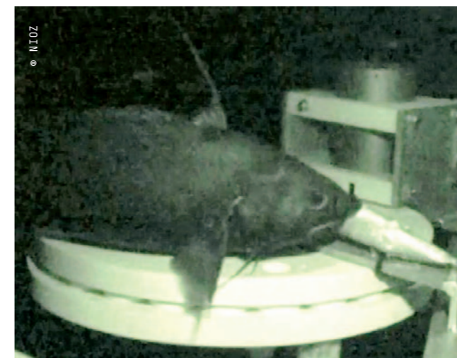
A CLOSE-UP of the deep-sea fish Antimora rostrata captured by time-lapse infrared camera mounted on the NIOZ ALBEX lander. The white disk below the fish, which is a bait dispenser, is 50 cm in diameter.
